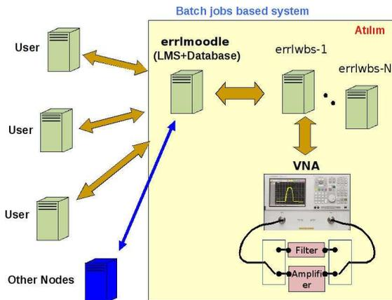
Figure 2. Batch job based ERRL system
