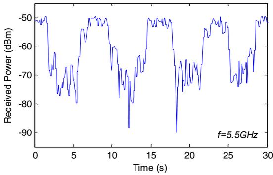
Figure 2. Received signal variation when radio link is continuously blocked by human body.
