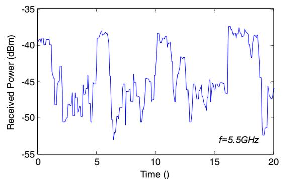
Figure 4. Received signal variation when radio link is continuously blocked by human body.
